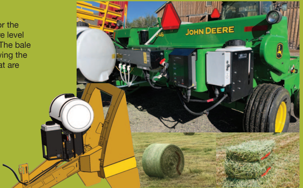
A food-grade stripe is applied to indicate higher moisture areas of the bale using the optional Dye Marker kits available for both Round and Small Square balers.
